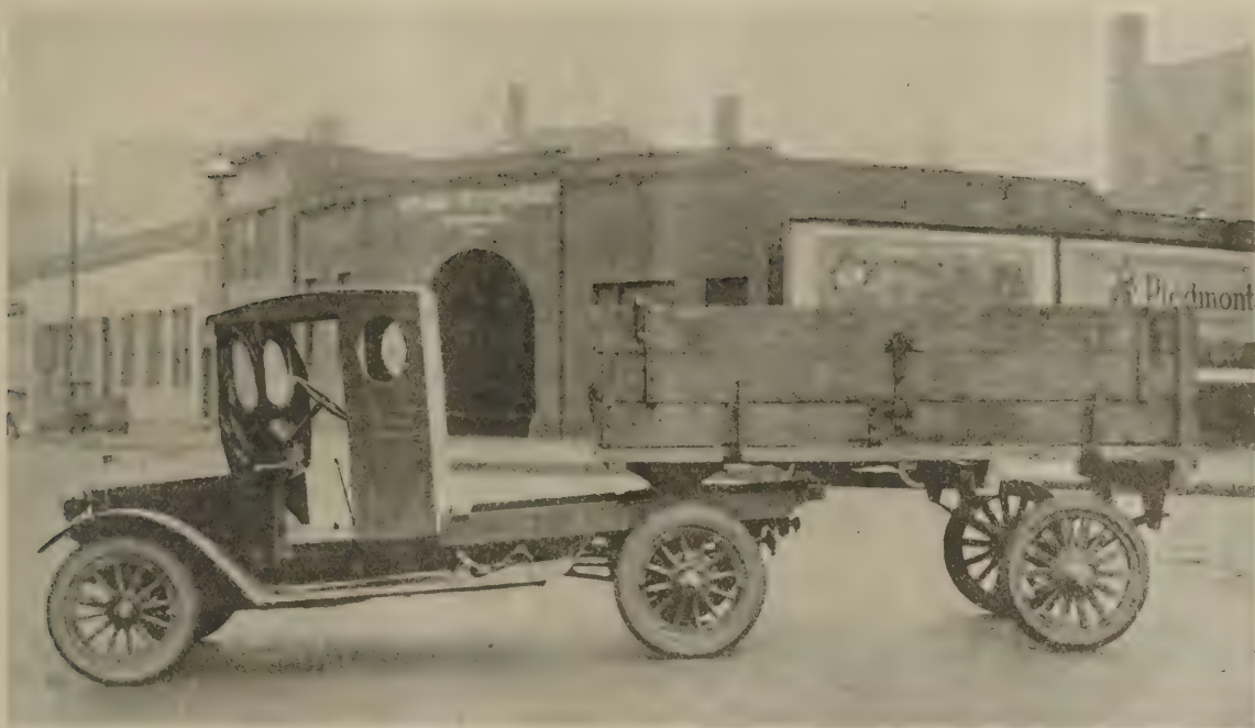
A \frac{3}{4} -ton speed wagon with rocking "fifth" wheel, used to haul brick
